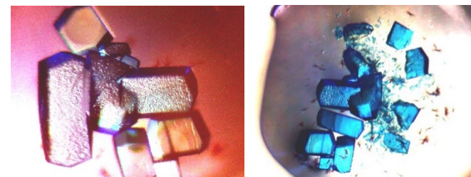
Figure 7: Left – Crystal from well B3 (methylene blue stain). Right – Crushed crystal from well B3 (methylene blue stain).
